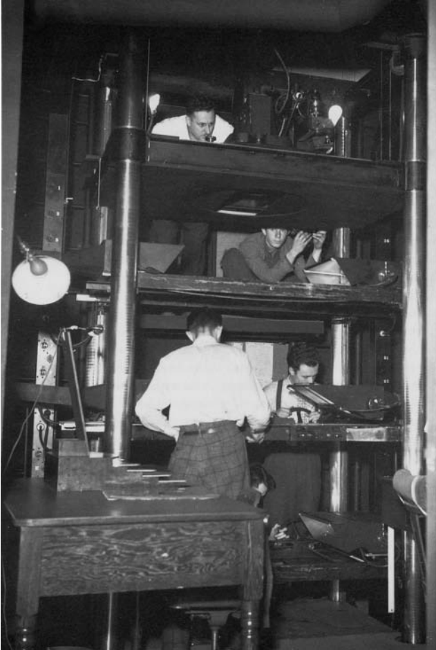
Figure 1.3 Disney multiplane camera
