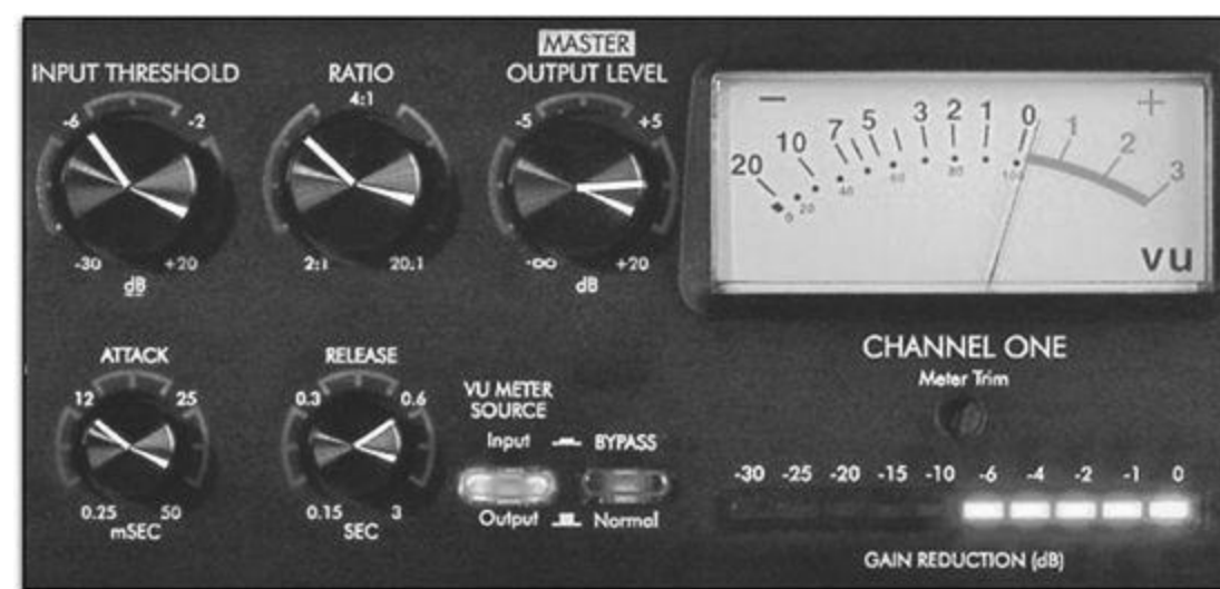
Figure 9.1 Typical compressor parameter controls.
