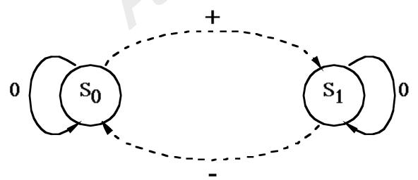
In this diagram, a dashed arrow represents a binary 0 and a solid arrow represents a binary 1. The labels –, 0, and + are used to indicate the line voltages: negative, zero, and positive, respectively.
