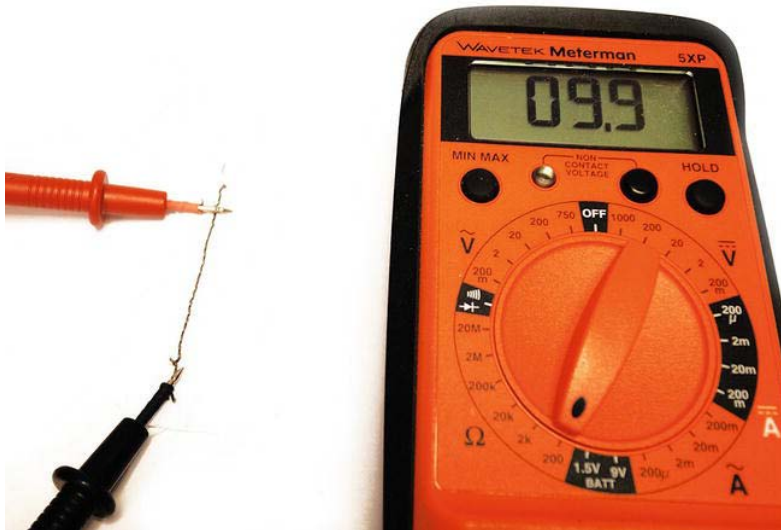
Figure 5-2. Checking for conductivity in the conductive thread
