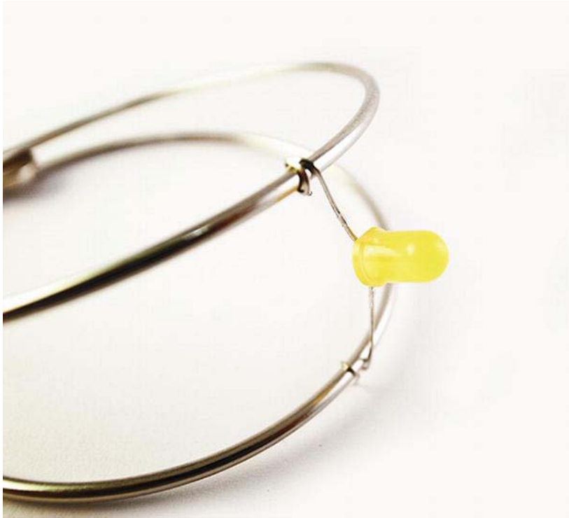
Figure 5-20. Wrapping the LED legs around the rings
