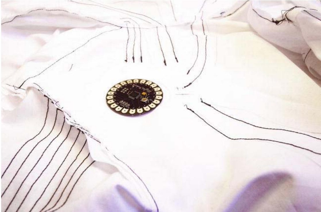
Figure 9-10. Connect all components back to the Arduino LilyPad
