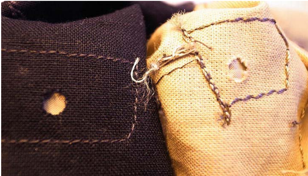
Figure 7-7. Conductive thread connections
