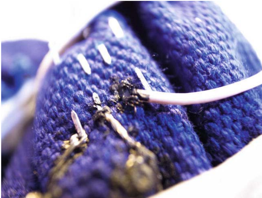
Figure 14-12. Paint the end connections with conductive ink to make them more secure.
