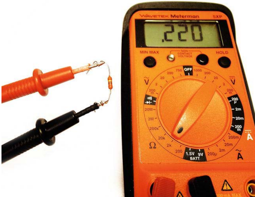
Figure 5-3. Measuring the resistance of a resistor
