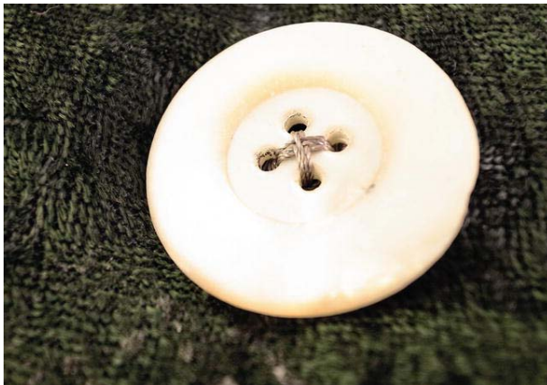
Figure 8-11. The button is stitched like a regular button using conductive thread.
