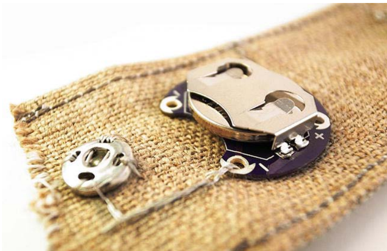
Figure 5-15. Ground connection from the battery holder to the button
