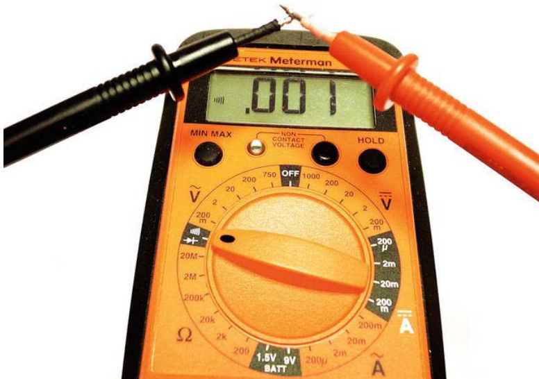
Figure 5-1. Finding conductivity with a multimeter
