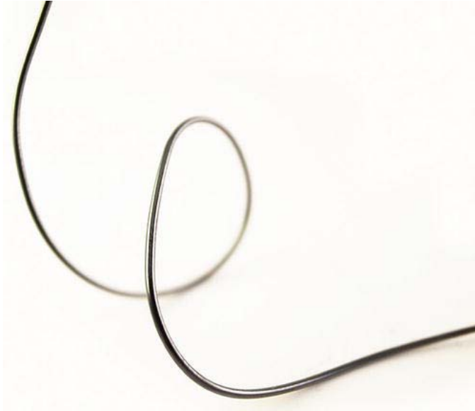
Figure 4-9. Smart wire that remembers shapes
