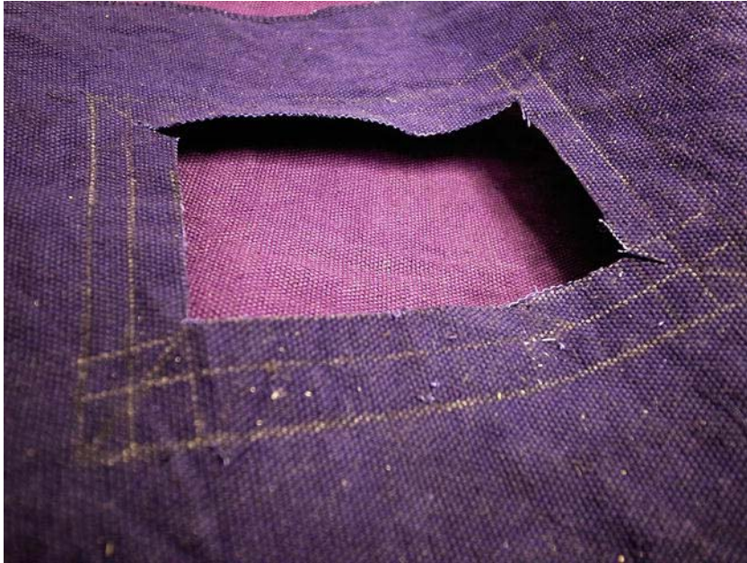
Figure 6-9. Hole cut for the solar panel with diagonal corner cuts
