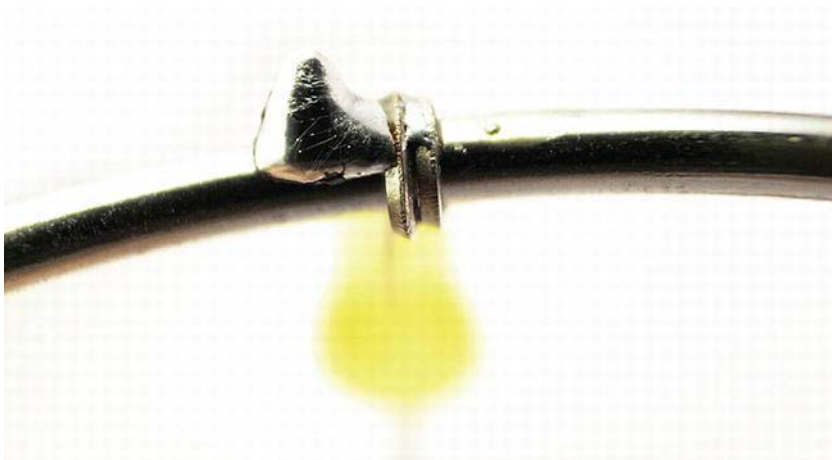
Figure 5-23. A cold soldering joint
