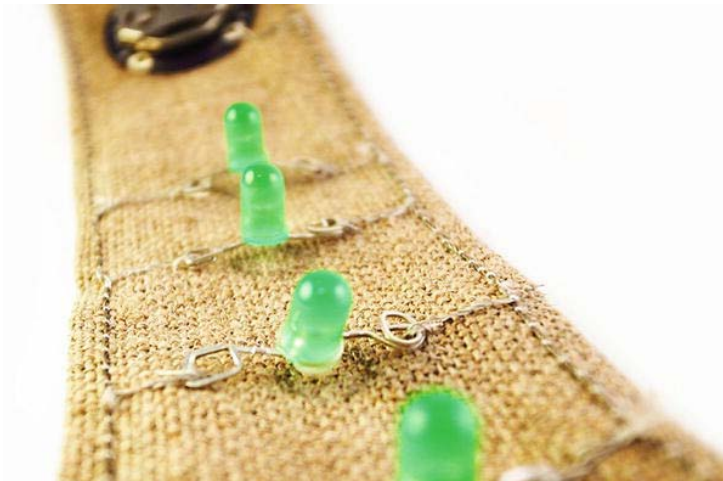
Figure 5-17. LED connected to each of the horizontal lines of conductive thread
