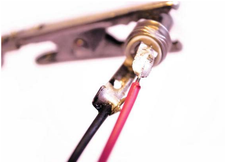
Figure 13-19. Soldering the DC connector
