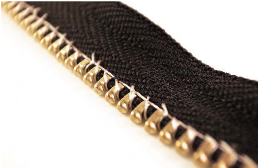
Figure 8-4. Making an extra run of thread under your stitching on the back side helps.
