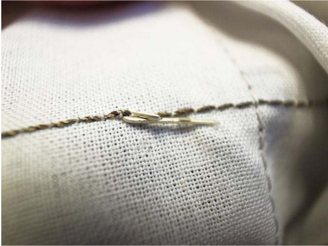
Figure 11-13. Securing the LED leg to the conductive thread line
