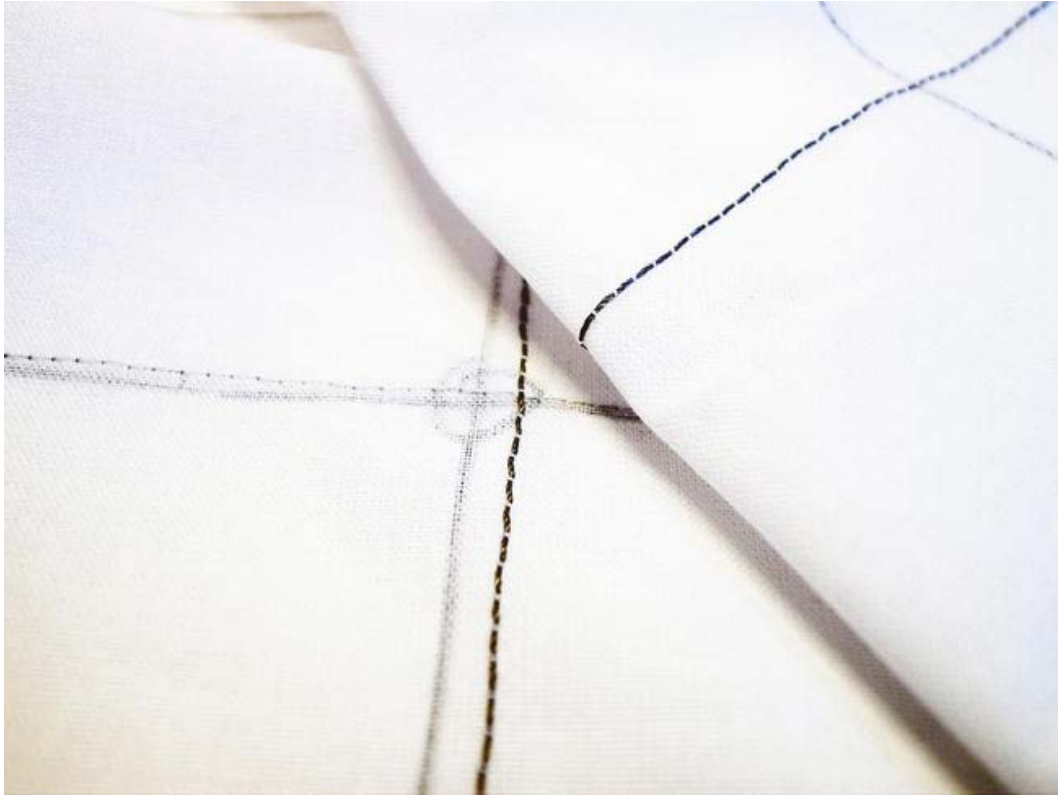
Figure 11-5. Conductive thread matrix
