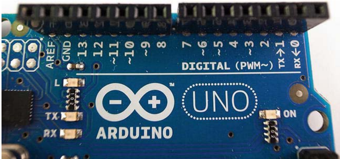
Figure 3-9. Digital pins from 0 to 13
