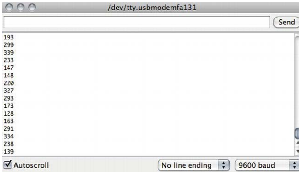
Figure 8-7. Serial monitor printing data
