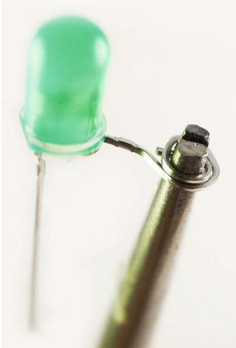
Figure 5-13. Modifying the LED legs
