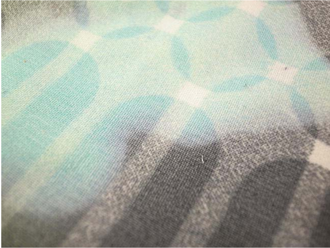
Figure 4-2. Thermochromic screen print after heat is applied
