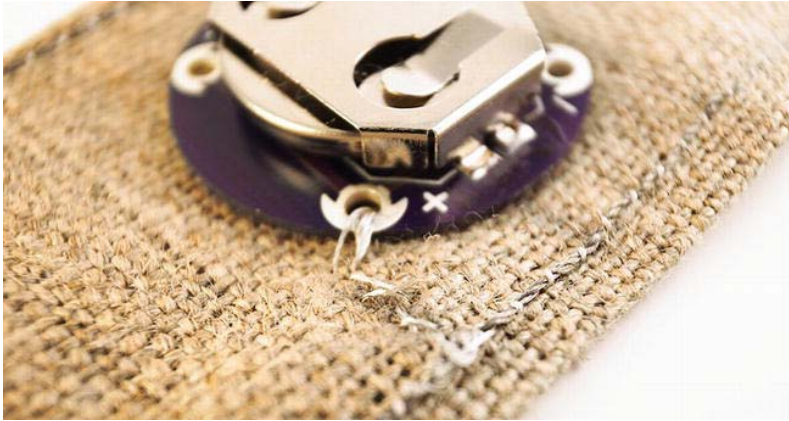
Figure 5-16. Making the power connection
