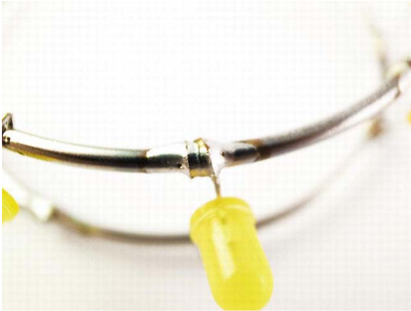
Figure 5-24. The solder should spread onto the material.
