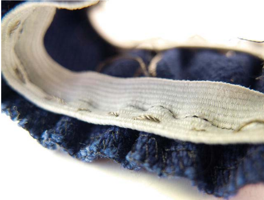
Figure 14-13. The extended ground connection between the battery and the ATtiny made with conductive thread into the elastic that connects to the skin
