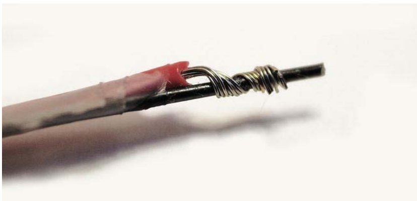
Figure 12-5. Attaching normal wire to the SMA wire
