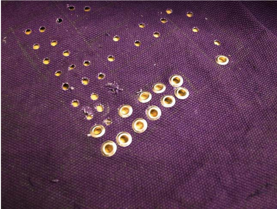
Figure 6-12. Eyelets punched in place
