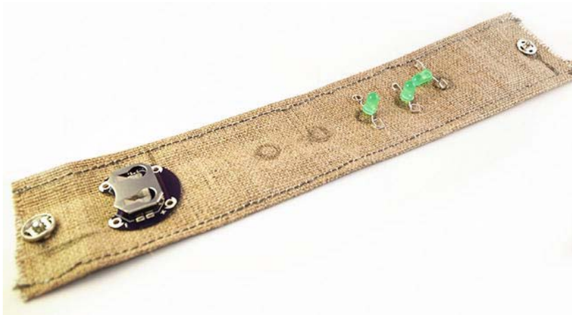
Figure 5-14. Marking the placement of components and needed connections
