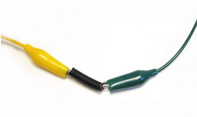
Figure 12-2. The SMA wire when it has reached the original position
