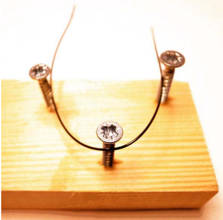
Figure 12-12. Reprogramming the SMA wire
