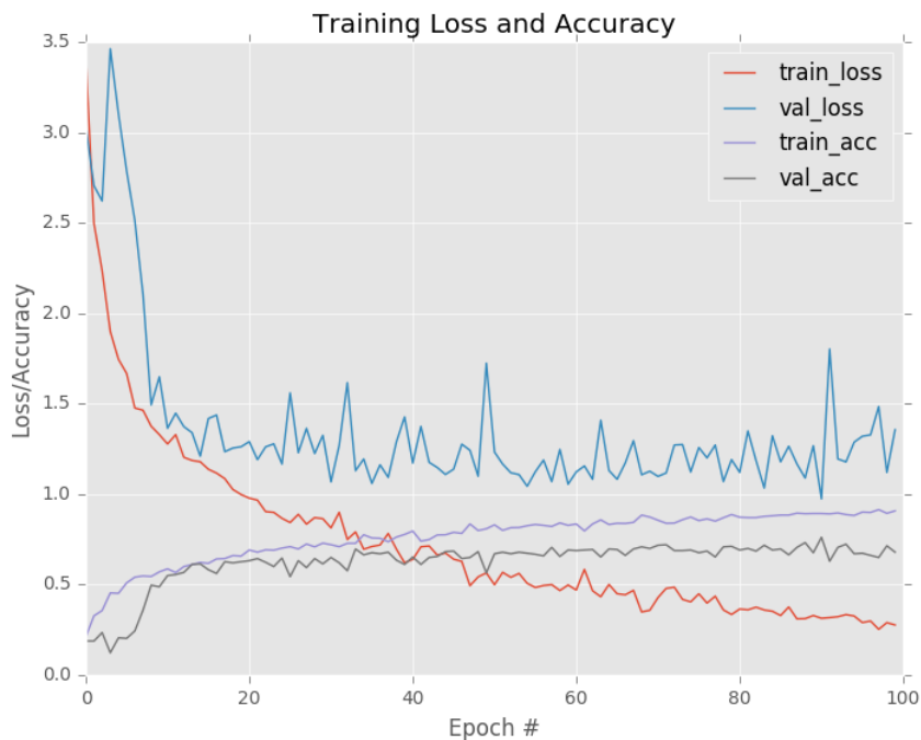
Figure 2.6: Applying MiniVGGNet to Flowers-17 with data augmentation. Overfitting is still a concern; however, we are able to obtain substantially higher classification accuracy and lower loss.
