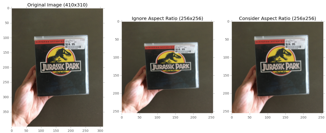
Figure 2.4: Left: The original input image ( 410 \times 310 ). Middle: Resizing the image to 256 \times 256 pixels, ignoring the aspect ratio. Notice how the image now appears squished and distorted. Right: Resizing the image to 256 \times 256 while maintaining the aspect ratio.
