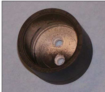
Cap showing drilled holes
