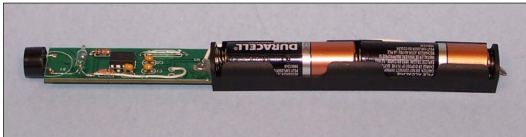
PCB and battery assembly
