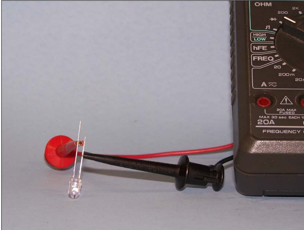
Finding the cathode with a meter
