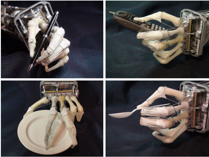
Fig. 7.5 Example postures illustrating the ACT Hand grasping several household objects. Particular attention was paid to the replication of human bone structure, including the weight of each finger element, and to the anatomy of the flexor/extensor tendon web. Note the natural appearance of each grasp posture, a consequence of faithfully modeling actual hand kinematics
