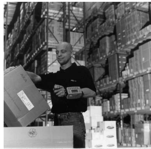
FIGURE 15.2. Symbol's WSS 1000 series wrist-mounted wearable computer with ring scanner.
