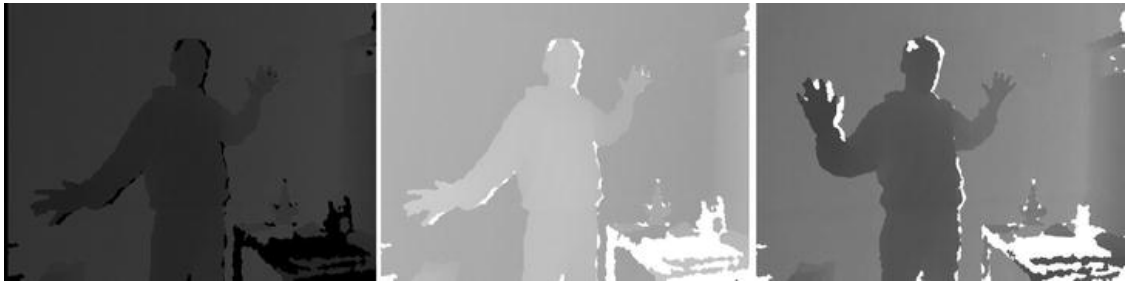
Figure 3-6. Different visualizations of the depth image—from left to right: raw depth image, depth image from Listing 3-7, and depth image from Listing 3-8
