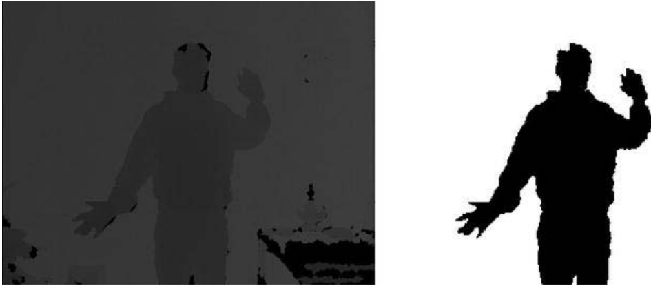
Figure 3-11. Raw depth image (left) and processed depth image with player indexing (right)
