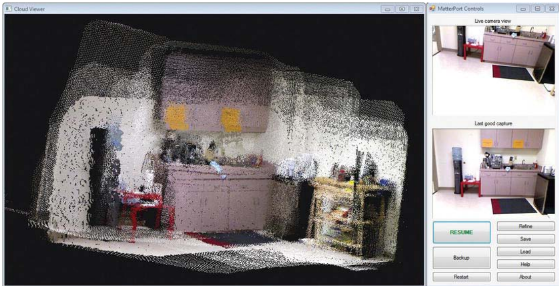
Figure 3-17. MatterPort showing a roughly aligned 3-D capture
