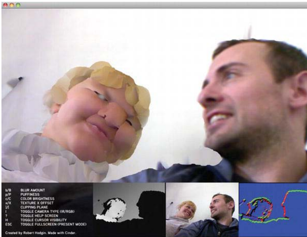
Figure 3-12. The Body Dysmorphia Toy applies puffiness to the user on the left within the range of depth sensor, but not to the user on the right who is too close to the sensor.
