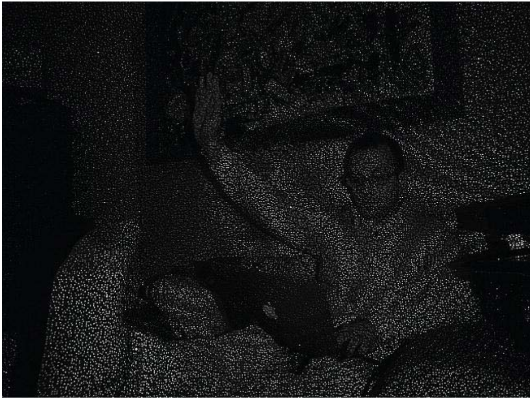
Figure 2-10. IR map image from Libfreenect. Speckled dots are projected on the scene from the IR projector.
