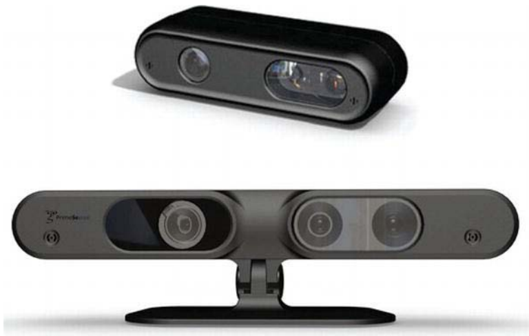
Figure 2-6. The original PrimeSense reference design, the PS1080 (top), and the newer design (bottom)
