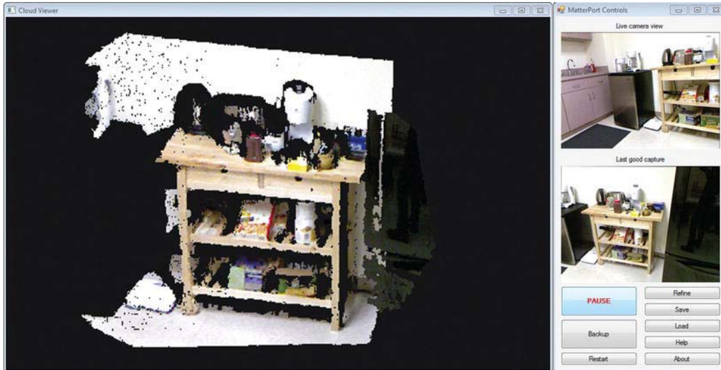
Figure 3-15. MatterPort Cloud Viewer window to the left of the control panel showing start of process with one good capture displayed
