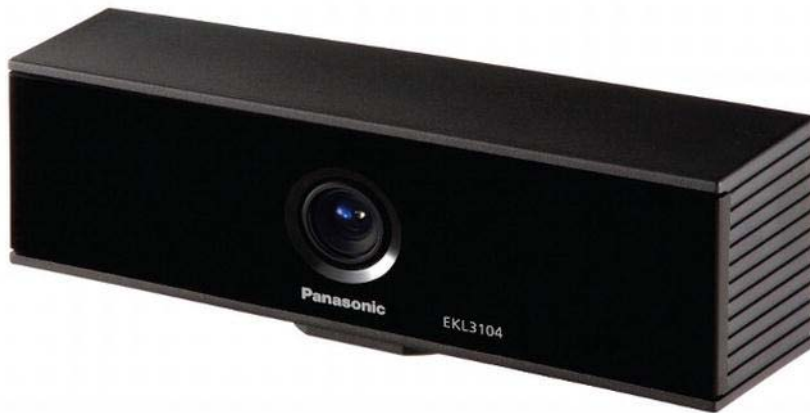
Figure 2-8. Panasonic D-Imager time-of-flight depth sensor with an array of near infrared LEDs hidden to the left and right of the lens.
