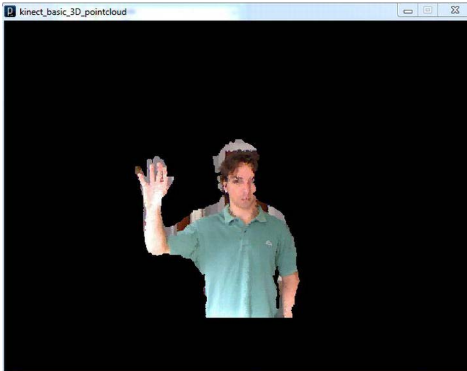
Figure 4-9. Thresholding example, with a poorly calibrated Kinect
