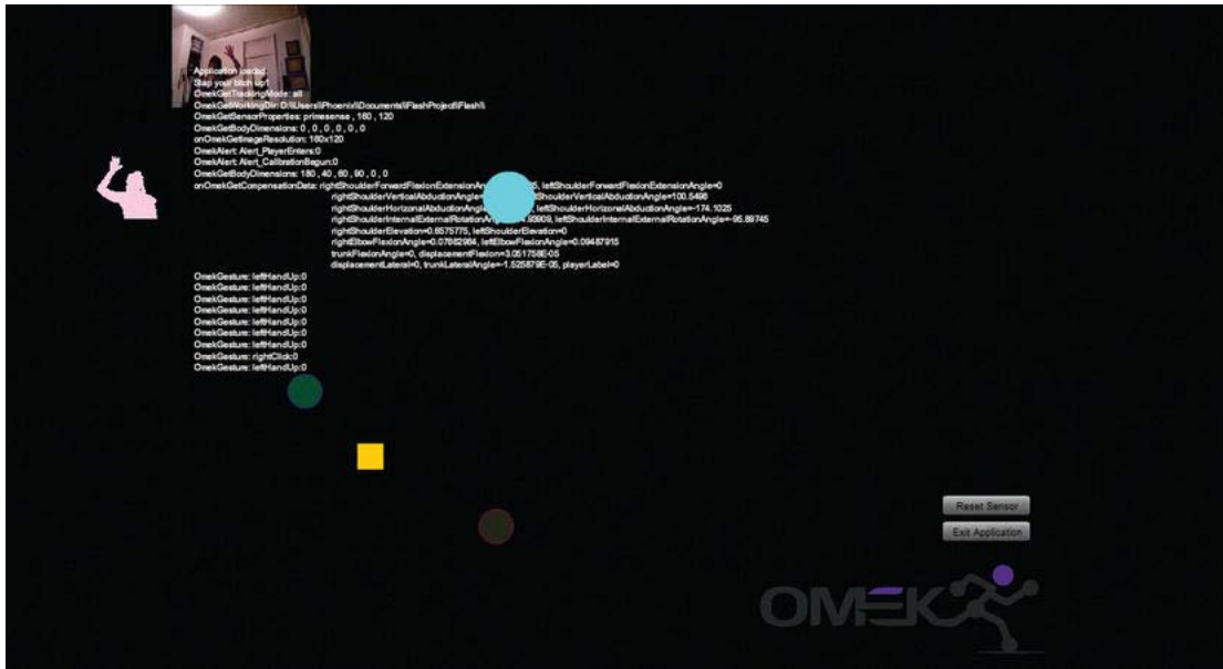
Figure 6-9. Beckon registering the leftHandUp gesture and moving a box to the location of my left finger tip where on screen the gesture was performed.
