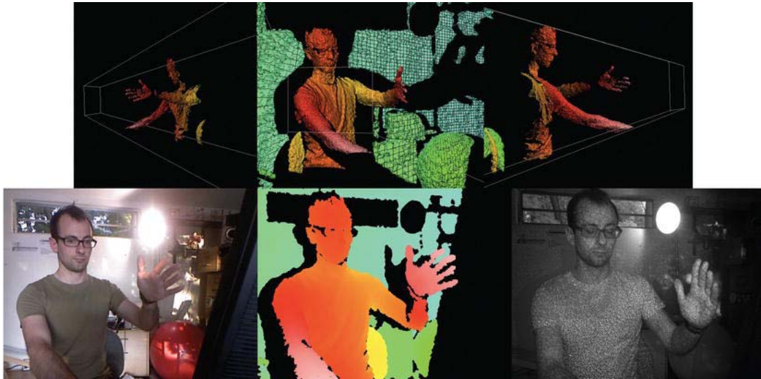
Figure 2-12. Upper row, point cloud rotated to show alternate viewpoints. Lower row, source RGB, depth, and IR map images for point cloud scene.
