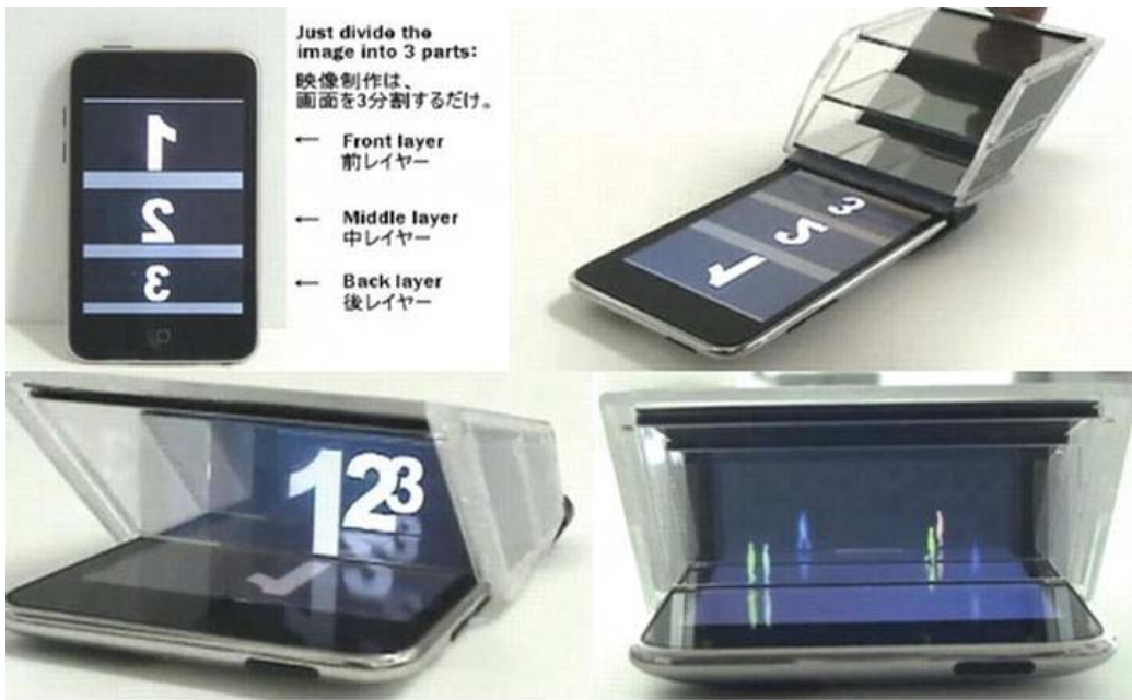
Figure 9-7. The i3Dg accessory for iPhone utilizes three panes of plastic to create a multi-depth experience, utilizing the principle of Pepper’s Ghost. Image courtesy i3Dg
