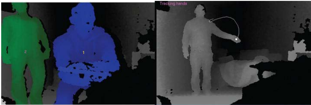
Figure 2-13. Left, user segmentation tracking two people. Right, demonstration of a point tracking a hand
