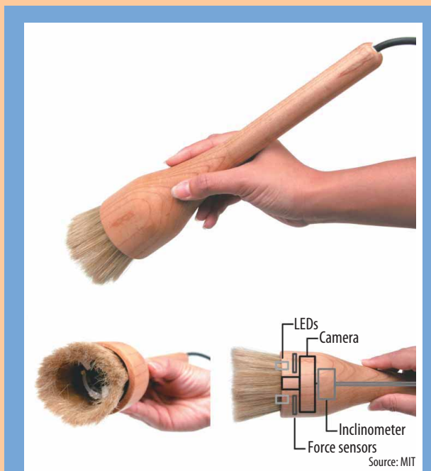
Researchers have built a high-tech brush that lets artists pick up images, video, audio, colors, and textures from objects and paint them onto a touch-screen canvas.
