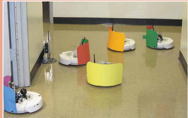
Figure A. Convoy of four robots following a leader. The red robot leaves the group to charge its battery at a base station.
