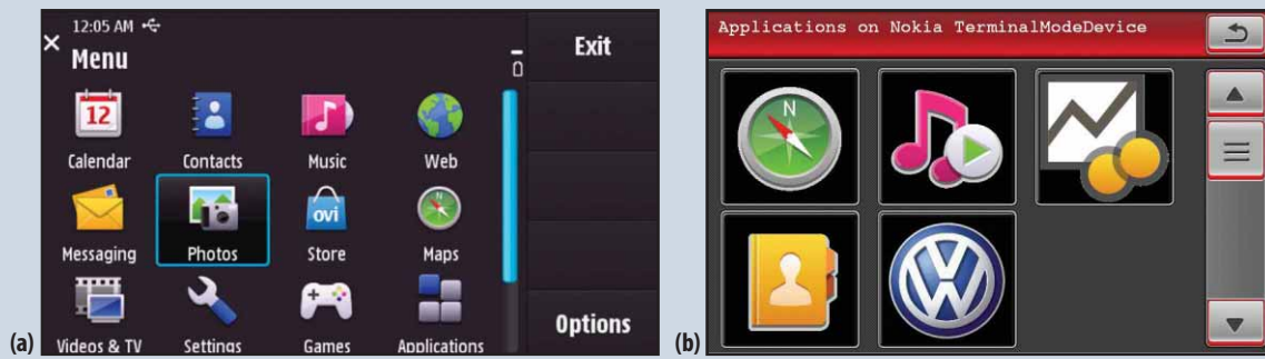
Figure 4. Native phone versus car mode user interface: (a) smartphone application menu, (b) customized menu generated by in-vehicle infotainment system.
