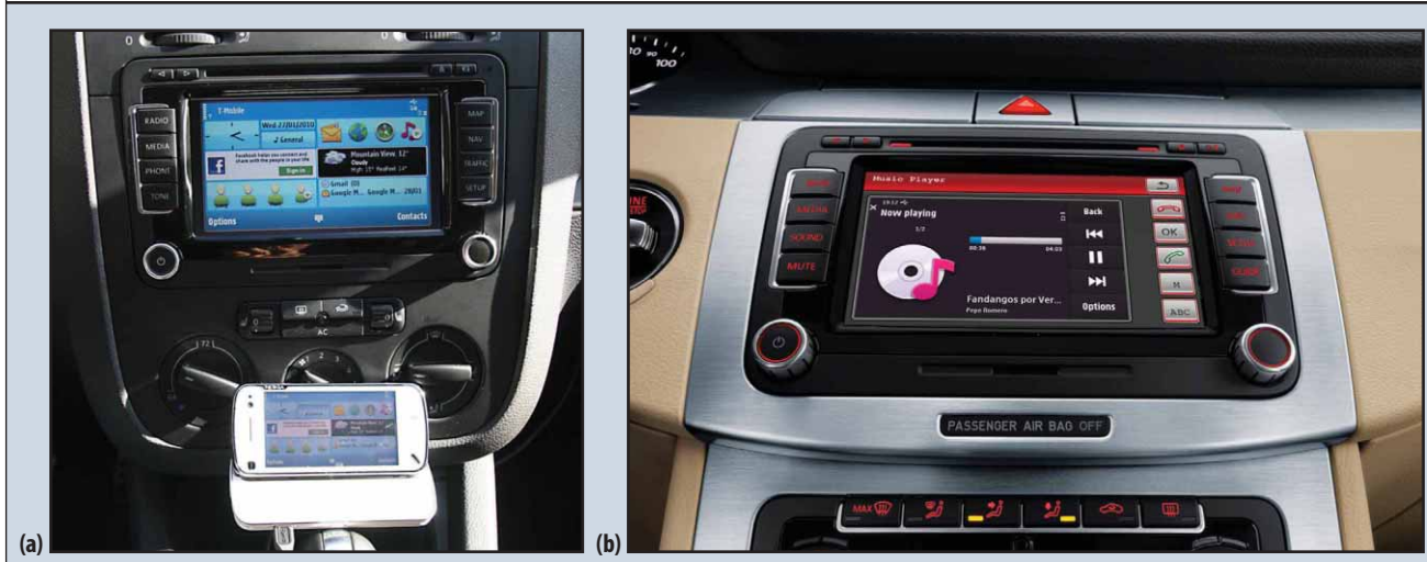
Figure 2. Music Player interface. (a) Smartphone connected via Terminal Mode and (b) head unit touch screen displaying the Music Player application.
