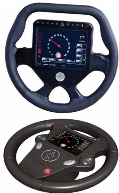
Figure 2. Intelligent steering wheel (ISW) developed by AUDIO MOBIL Elektronik GmbH. This prototype is equipped with an integrated touch screen that visualizes instrument panel, infotainment, and navigation information. All cockpit controls—turn indicator, light switch, and so on—are fully integrated into the steering wheel and can be activated via either the touch screen or buttons at the top of the wheel. The ISW ensures short distances for both input and output.
