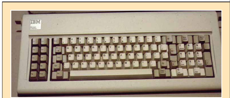
Figure 2. IBM PC original keyboard. The single instances of Ctl and Alt are on the left side of the keyboard, and the single instance of Del is on the far right, providing a set of keys that would be difficult to hit by accident.
