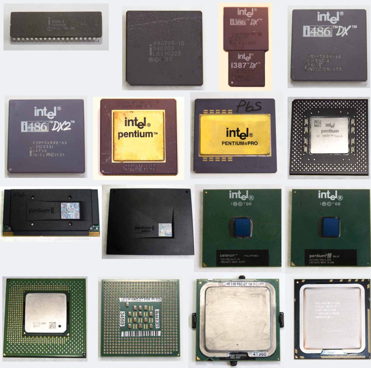
Figure 2. Sample of Intel's IBM PC-compatible processors over three decades. Top row: 8088 to 80486; second row: 80486DX2 to Pentium MMX; third row: Pentium II and Xeon modules, Celeron, and Pentium III; fourth row: Pentium IV to Core i7.
