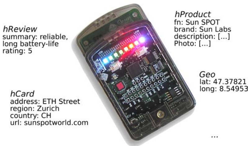
Fig. 5.10 Compound Microformats for Describing a Sun SPOT Using the Geo, hCard, hProduct and hReview Microformats
