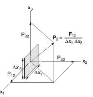
**Fig. 4.3.** Stress  $\mathbf{P}_2$ , defined as force per unit area, on a small surface perpendicular to the  $x_2$  axis. Its components along the three axes are, respectively,  $P_{12}$ ,  $P_{22}$ ,  $P_{32}$
