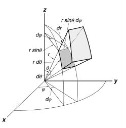
**Fig. 3.4.** Differential elements in the spherical coordinates. The differential length in the direction of increasing  $\theta$  is  $r d\theta$ . The differential length in the direction of increasing  $\varphi$  is  $r \sin \theta d\varphi$ . The differential volume element is  $r^2 \sin \theta dr d\theta d\varphi$
