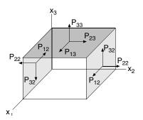
Fig. 4.4. The nine components of a stress tensor at a point can be represented as normal and tangential forces on the surfaces of an infinitesimal cube around the point
