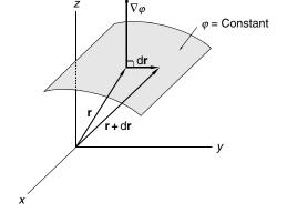
Fig. 2.6. Gradient of a scalar function.  $\nabla \varphi$  is a vector normal to the surface of  $\varphi = \text{constant}$
