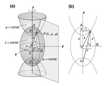
Fig. 3.7. Elliptical Coordinate System. (a) The coordinate surfaces generated by an ellipse, two hyperbolas and a plane containing the major axis of the ellipse. (b) The confocal ellipse given by  $r_2 + r_1 = \text{constant}$ , and the confocal hyperbolas given by  $r_2 - r_1 = \text{constant}$
