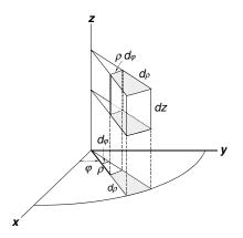
**Fig. 3.2.** Differential elements in cylindrical coordinates. Note that the differential length in the direction of increasing  $\varphi$  is  $\rho d\varphi$ . The differential volume element is  $\rho d\varphi d\rho dz$ .
