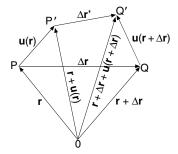
Fig. 4.6. The strain of a deformed elastic body. The body is strained if the relative distance of two nearby points is changed. The strain tensor depends on the variation of the displacement vector  $\mathbf{u}$  with respect to the position vector  $\mathbf{r}$
