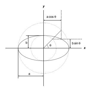
Fig. 3.8. Parametric form of an ellipse. Parametrically an ellipse can be written as  $x = a \cos \theta$ ,  $y = b \sin \theta$
