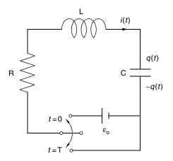
Fig. 6.7. A RLC circuit. The open circuit without charge on the capacitor is closed at t = 0. At t = T, the battery is removed from the circuit in such a way that the circuit is closed but without emf
