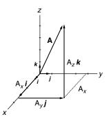
**Fig. 1.10.** Vector components. **i**, **j**, **k** are three unit vectors pointing in the direction of positive x-, y- and z-axis, respectively.  $A_x$ ,  $A_y$ ,  $A_z$  are the projections of **A** on these axes. They are components of **A** and  $\mathbf{A} = A_x \mathbf{i} + A_y \mathbf{j} + A_z \mathbf{k}$
