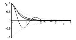
**Fig. 5.2.** Free vibrations with viscous damping. Initially the block is at  $x_0$  and released from rest. The *dotted line* is for the over damped motion, the *line of open circles* is for the critically damped motion, the *solid line* is for the under damped motion. The damped amplitude is shown as *dashed lines*
