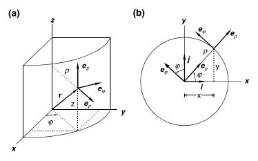
**Fig. 3.1.** Cylindrical coordinates. (a) A point is specified by  $(\rho, \varphi, z)$ , the unit vectors  $\mathbf{e}_{\rho}, \mathbf{e}_{\varphi}, \mathbf{e}_{z}$  are pointing in the direction of increase of the corresponding coordinates, (b)  $\mathbf{e}_{\rho}, \mathbf{e}_{\varphi}$  are moved to the origin to find the relationships with  $\mathbf{i}, \mathbf{j}$  of the rectangular coordinate system
