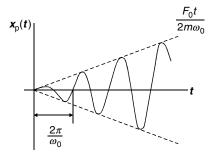
Fig. 5.5. Resonance without damping. When the forcing frequency coincide with the natural frequency, the motion will become unbounded
