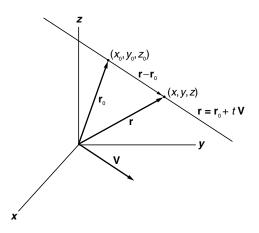
Fig. 1.17. A straight line in the parametric form
