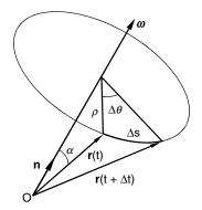
Fig. 2.2. Angular velocity vector  $\boldsymbol{\omega}$ . The velocity  $\mathbf{v}$  of a particle moving around a circle is given by  $\mathbf{v} = \boldsymbol{\omega} \times \mathbf{r}$
