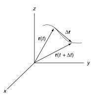
Fig. 2.1. The tip of **r** traces out the trajectory of a particle moving in space,  $\Delta \mathbf{r}$  is independent of the origin
