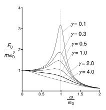
**Fig. 5.6.** Forced vibration with viscous damping. Amplitude of the steady-state as a function of  $\omega/\omega_0$ ,  $\gamma = (c/m\omega_0)^2$  represents the strength of damping. For  $\gamma \geq 2$ , there is no maximum
