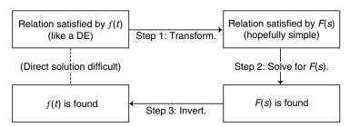
Fig. 6.1. Steps of using Laplace transform to solve differential equations
