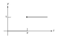
**Fig. 6.3.** The Heaviside unit step function u(t-c)
