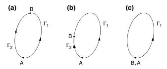
Fig. 2.8. Path independence of the line integral of  $\nabla \varphi \cdot d\mathbf{r}$ . (a) The value of the integral from A to B along  $\Gamma_1$  is the same as along  $\Gamma_2$ . (b) They are still the same even though  $\Gamma_2$  is much shorter. (c) As  $\Gamma_2$  shrinks to zero, the integral along  $\Gamma_2$  vanishes. The integral along  $\Gamma_1$ , which becomes a loop integral, must also be zero
