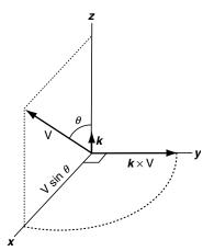
Fig. 1.13. The cross product of  $\mathbf{k}$ , the unit vector along the z-axis, and  $\mathbf{V}$ , a vector in the *xz*-plane
