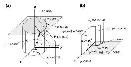
Fig. 3.5. Coordinate surfaces and coordinate curves of cylindrical coordinate system. (a) The side surface of the cylinder ( $\rho = \text{constant}$ ), the horizontal plane (z = constant), and the plane containing z axis ( $\varphi = \text{constant}$ ) are the coordinate surfaces. The intersections of them are the coordinate curves. (b) Locally, the three unit vectors along the coordinate curves form an orthogonal basis set
