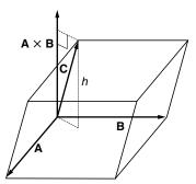
Fig. 1.16. The volume of the parallelopiped is equal to the triple scalar product of its edges as vectors
