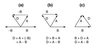
**Fig. 1.3.** Subtraction of two vectors: (a) as addition of a negative vector; (b) as an inverse of addition; (c) as the tip-to-tip vector which is the most useful interpretation of vector subtraction
