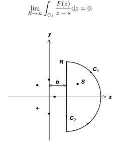
Fig. 6.11. The first contour used to obtain the complex inversion of the Laplace transform
