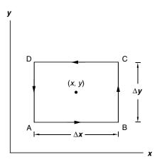
**Fig. 2.16.** The line integral of  $\mathbf{A} \cdot d\mathbf{r}$  around the four sides of the infinitesimal square is equal to the surface integral of  $\nabla \times \mathbf{A}$  over the area of this square
