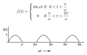
Fig. 6.9. Half-wave rectifier. The definition over one period is  $f(t) = \sin \omega t$  for  $0 < t < \pi/\omega$  and f(t) = 0 for  $\pi/\omega < t < 2\pi/\omega$
