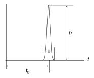
**Fig. 6.2.** A sharply peaked function. If  $h \to \infty$  and  $\tau \to 0$  in such a way that the area under it is equal to 1, then this function becomes a delta function  $\delta(t - t_0)$
