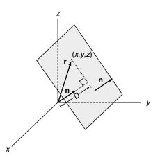
**Fig. 1.18.** A plane in space. The position vector  $\mathbf{r}$  from the origin to any point on the plane must satisfy the equation  $\mathbf{r} \cdot \mathbf{n} = D$  where  $\mathbf{n}$  is the unit normal to the plane and D is the perpendicular distance between the origin and the plane
