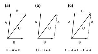
Fig. 1.2. Addition of two vectors: (a) connecting the tail of **B** to the tip of **A**; (b) connecting the tail of **A** to the tip of **B**; (c) parallelogram law which is valid for both free and bound vectors
