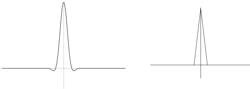
Figure 4.1: Left: Part of the graph of e^{-x^2} \text{sinc}(x) . Right: Part of the graph of the “hat” function. Both curves have maximum value 1, and two roots nearest 0 at x = -1 and x = +1 .
