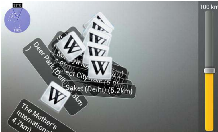
Figure 9-5. Several markers converge due to the compass going haywire next to a metallic object.
