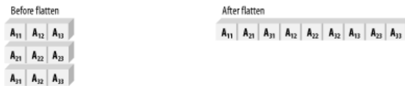
Figure 12-4. Memory representation of flat arrays
