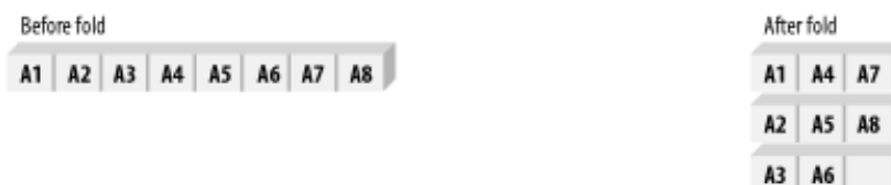
Figure 12-3. Memory representation of folded arrays
