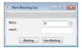
This application will calculate the Nth Fibonacci number specified by the first field. Using a number of 35 or higher will take from many seconds to several minutes to calculate by using the SlowFib function. Clicking on either of the two buttons will result in the same SlowFib function being called, and ultimately the same result being generated. So with this in mind, let's jump to the BlockingPanel's OnButton method to see what happens differently between the two buttons.
