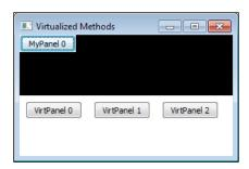
In each version of our Panel class we override the AddChild method, which is called every time that a window has a new child window created. AddChild is called inside the C++ part of the class when this happens, so in order to be able to override the method in our Python version of the class, we need to use the special version that provides access to overriding the virtualized method from the C++ class.
