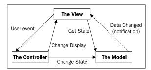
MVC is really one big monster pattern made up of other, simpler patterns working together. The Model implements an observer pattern to keep interested parties updated on changes, which allows it to be implemented separately from the View and Controller. The View and the Controller, on the other hand, implement a strategy pattern where the Controller is a strategy that implements the behavior of the View.
