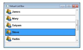
Our custom VListBox control could be used in any kind of application that wants to display a list of users. The constructor takes a list of usernames and calls SetItemCount to tell the control how many items it needs to be able to display. We also loaded a bitmap to use in our list's items. This bitmap is available in the sample code that accompanies this topic.
