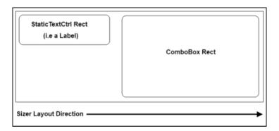
This diagram illustrates an alignment issue that can occur when some controls have a different-sized rectangle than the one next to it. This is a realistic example of a problem that can occur on GTK (Linux), as its ComboBoxes tend to be much taller than a StaticTextCtrl. So where on other platforms these two controls may appear to be properly center-aligned, they will look like this on Linux.
