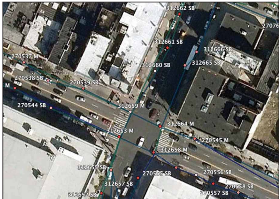
Figure 3. Image from a visualization tool that displays the underground electrical grid’s geometry superimposed on Google Earth satellite images. Each circle is a manhole, and each line between two manholes represents underground low-voltage cables connecting them.
