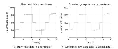
Fig. 14.1 Example 1D raw gaze *x*-coordinate data captured over a calibration validation grid: **b** Shows the effect of applying the Butterworth filter to the unfiltered data shown in (**a**) Notice in particular the removal of a downward spike at about the 16 s mark
