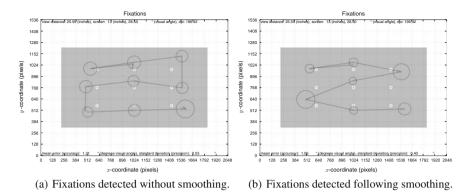
**Fig. 14.3** Example fixation data captured over a calibration validation grid: **b** shows the effect of applying the Butterworth filter prior to velocity-based fixation detection. **a** Shows the effect of not applying the Butterworth filter prior to velocity-based fixation detection. Notice how the bottom-left fixations points get averaged into one fixation
