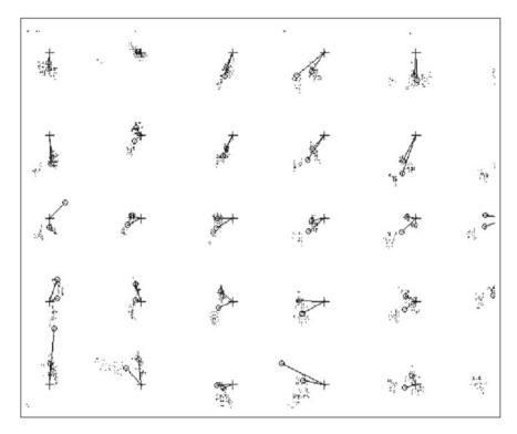
Fig. 8.4 Composite calibration data showing eye tracker slippage
