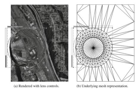
Fig. 19.13 The Pliable Display Technology (PDT) fisheye lens
