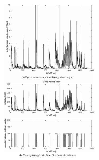
Fig. 13.9 Eye movement signal and filter responses
