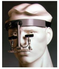
(c) Another example of infra-red limbus tracker apparatus, as worn by subject. Courtesy of Microguide, Downers Grove, IL <http://www.eyemove.com>. Reproduced with permission.
