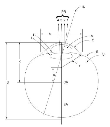
Fig. 5.7 Purkinje images. Reprinted in adapted form from Crane (1994) courtesy of Marcel Dekker, Inc. ©1994
