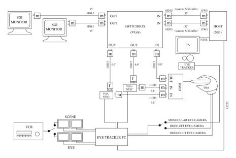
Fig. 6.2 Video signal wiring of the VRET lab at Clemson University
