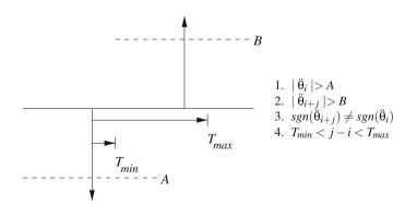
Fig. 13.8 Acceleration thresholding
