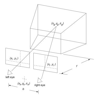
Fig. 7.4 Basic binocular geometry
