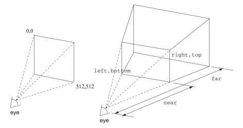
Fig. 7.1 Eye tracker to VR mapping
