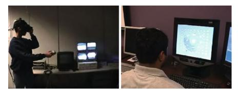
Fig. 19.1 Head-mounted and desktop (binocular) eye trackers
