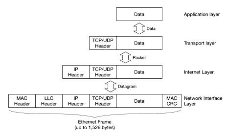
Fig. 13.6 Data format in TCP/IP layers
