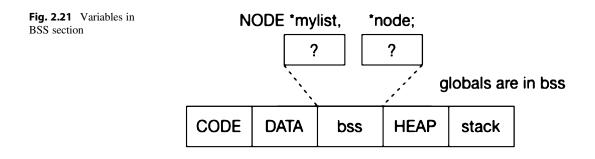
**Example C2.3:** The example program C2.3 builds a link list in the program's heap area but with individually allocated nodes.
