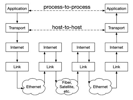
Fig. 13.2 Data flow paths in TCP/IP networks
