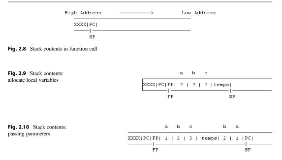
For this example, there are 3 automatic local variables, int a, b, c, each of sizeof(int) = 4 bytes. After entering main(), the stack contents becomes as shown in Fig. 2.9, in which the spaces of a, b, c are allocated but their contents are yet undefined.
