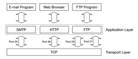
Fig. 13.5 Applications using TCP
