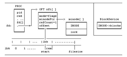
Fig. 11.14 Data structures for write
