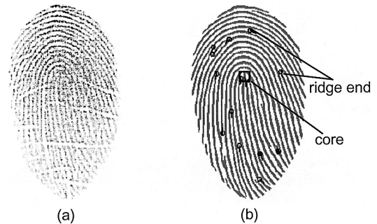
Fig. 10 Typical snapshots of the minutiae-based matching algorithm: (a) gray-scale normalization of a fingerprint image and (b) extraction of minutiae points (i.e., cores, deltas and ridge ends) after binarizing the fingerprint image.
