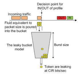
Fig. 4. Leaky bucket operation.
