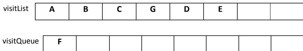
Gambar 31.8 Langkah 7 Algoritma Traversal Graph : BFS
